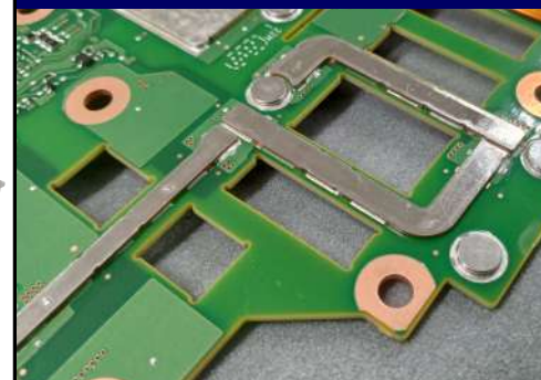
放熱対策(基板裏) Heat dissipation measures (Back side)
