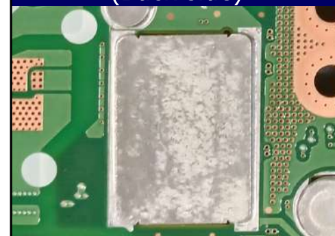
放熱対策(基板裏) Heat dissipation measures (Back side)
