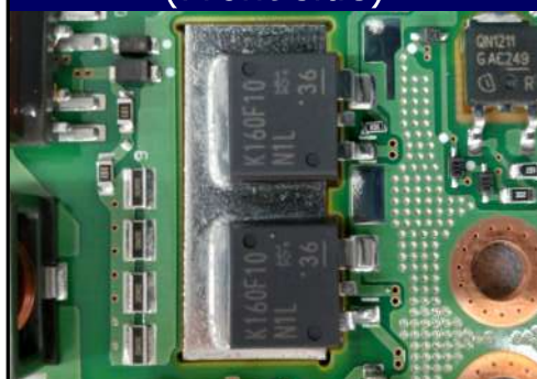
放熱対策(基板表) Heat dissipation measures (Front side)
