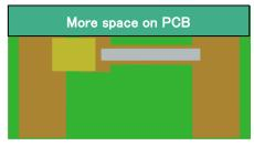
Use of pattern wiring reinforcing terminals allows for high currents in a narrow pattern, and is also effective in increasing the effective space and saving space on PCB.
